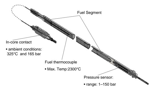
FIG. 3. Cut out view of re-instrumented fuel rod showing placement of fuel centre thermocouple and internal rod pressure sensor.
