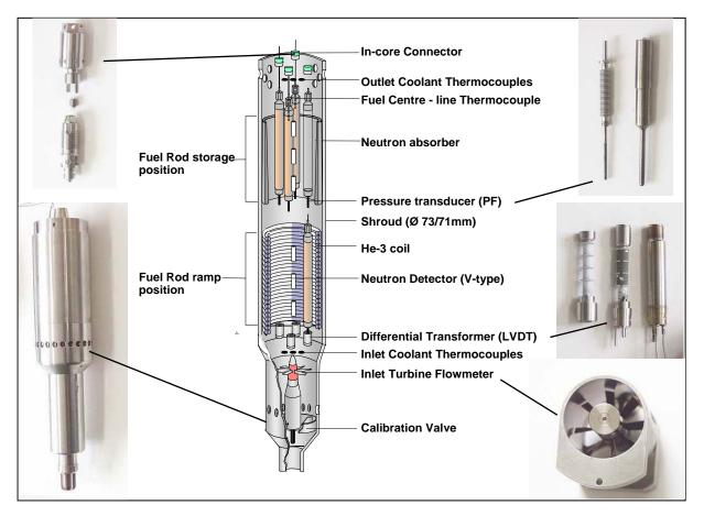
FIG. 2. Example of instrumentation available for a fuel power ramp test assembly in the Halden Reactor.
