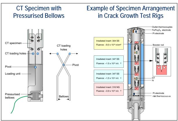
FIG. 4. Example of IASCC test rig. Crack growth is measured on-line with varying radiation levels, water chemistry and stress.
