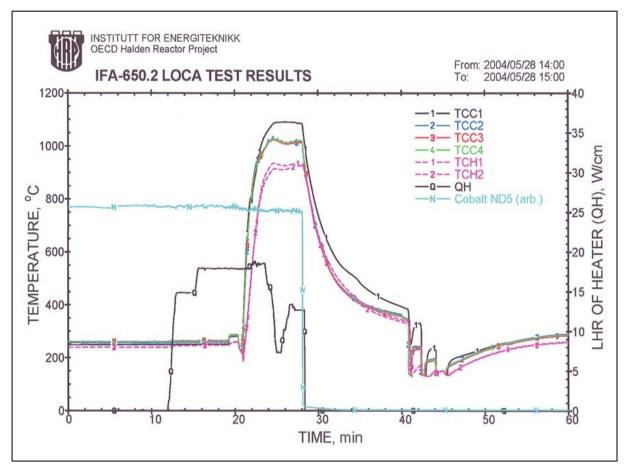
FIG. 5. Temperature measurements from LOCA test assembly.
