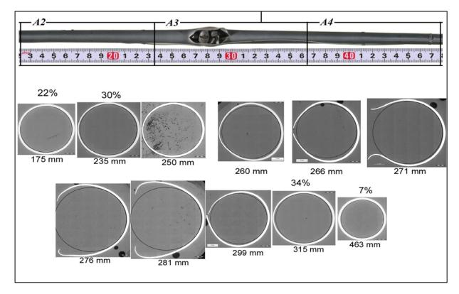
FIG. 6. Picture of clad burst with accompanying cross sections for a LOCA test.
